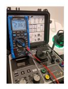
Versatile True RMS multimeter with dual display for displaying two signals simultaneously.
